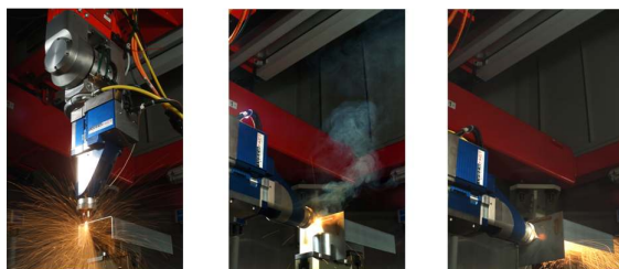
1. Trimming the profile and recording height coordinates
