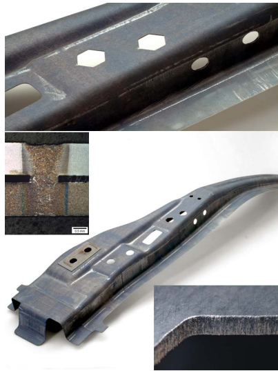
Fig. 7: Combi-processed B-pillar with cross-section of the welded reinforcing sheet and details of the cut contours, max. laser beam power 2.5 kW.
