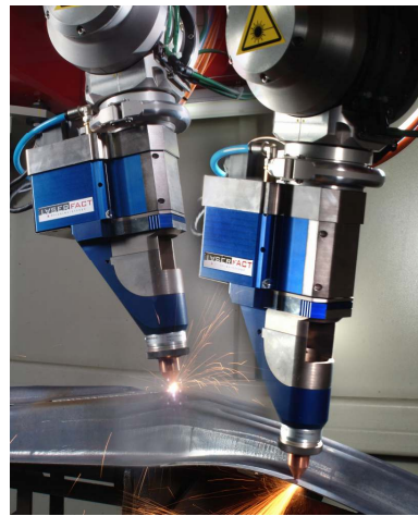
Fig. 8: Combi-head at work. Cutting and welding process on the B-pillar with a gantry-robot (photo: multiple exposures).
