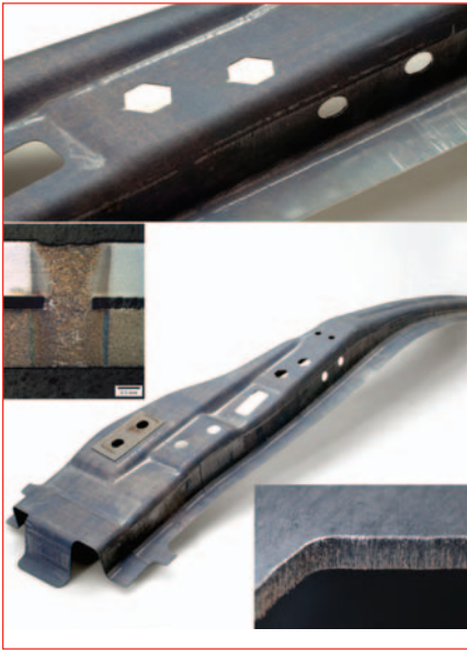
Fig. 5 — Combi-processed B-pillar with cross section of the welded reinforcing sheet and details of the cut contours. Maximum laser beam power is 2.5 kW.
